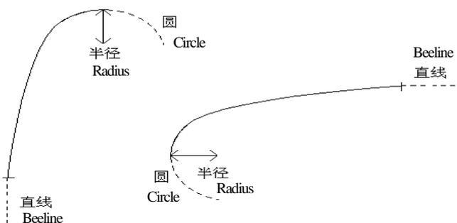
Press the button CUR in main line input process screen and you can define the curve which comprises the minimum radius and arc length. The definition of positive and negative radius is the same as the arc. Similarly, its arc length shall not be negative.
