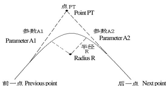
Press the button PT in main line input process screen and you can define the point which comprises coordinates, radius as well as A1 and A2 parameters of the curve. The radius, A1 and A2 shall not be negative. If radius is entered, an arc of specified radius will be inserted between current point and next point. If parameters of the curve A1 and A2 are entered, a curve of specified length will be inserted between the beeline and the arc.
