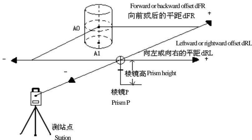
To measure coordinates of ground point A1, instrument height and prism height shall be set.
