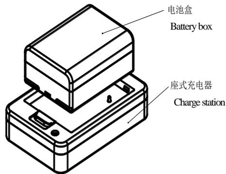
2. Insert one terminal of the transformer into the charge station and the other into the power socket-outlet. Red light of the transformer indicates charging is underway and, when it turns green, it indicates charging is finished.
