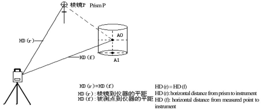
There are two ways to set vertical angle in angle offset measurement mode:
